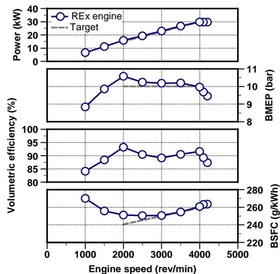
Figure 1 Tests results from the MAHLE range extender engine
