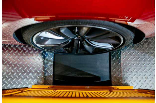
>> High specification 4WD chassis dyno
