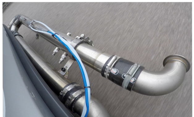
>> PEMS testing in vehicle
