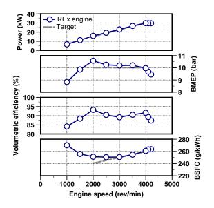
Figure 1 Tests results from the MAHLE range extender engine
